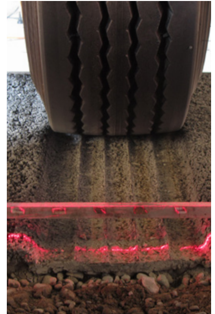
Section through basecourse sample showing tyre, rut in asphalt surface and laser line measuring system.
